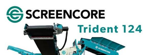
The Trident 124 is a compact scalper which delivers high production on heavy-duty applications yet folds small enough to transport without the need for a permit
